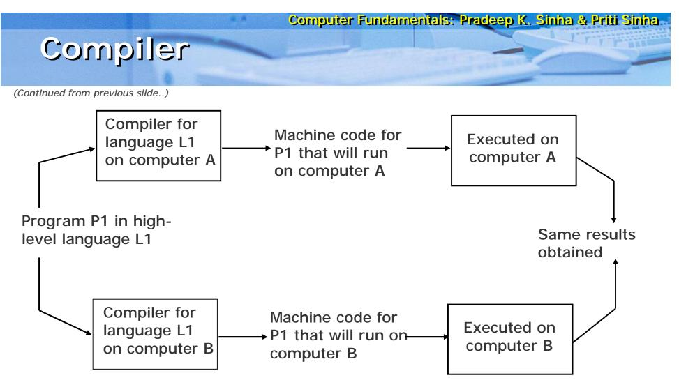
Illustrating the machine independence characteristic of a high-level language. Separate compilers are required for the same language on different computers
